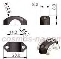
Part No. BG 8 - Cap Material: Nylon Weight of the cap only: 0.8 g
