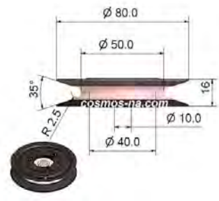
Part No. NT 019 Material: 95% Al 2 O 3 Bearing 6200 ZZ Wt. 96 g
