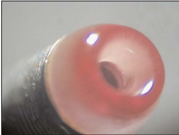
The exit orifice of a ruby needle guide, epoxy-bond to a stainless steel tube
